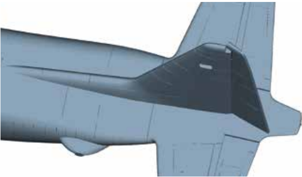
Rudder travel: 10-12mm left / 10-12mm right
