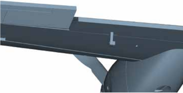
Ailerons travel: 10-12mm up / 10-12mm down
