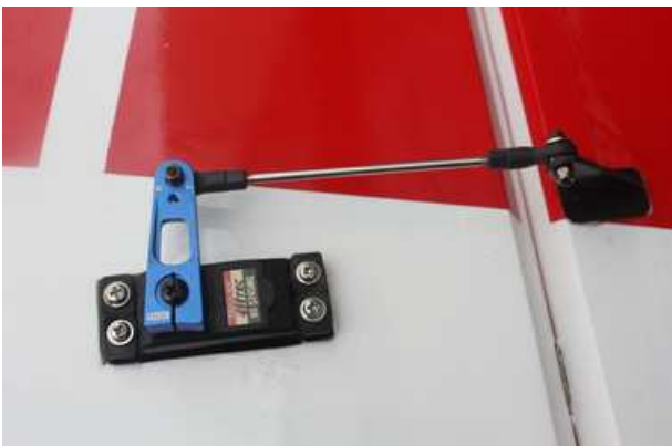
26mm/1in for aileron No. KAG0S70F/KAG0S70H/KAG0S70J
